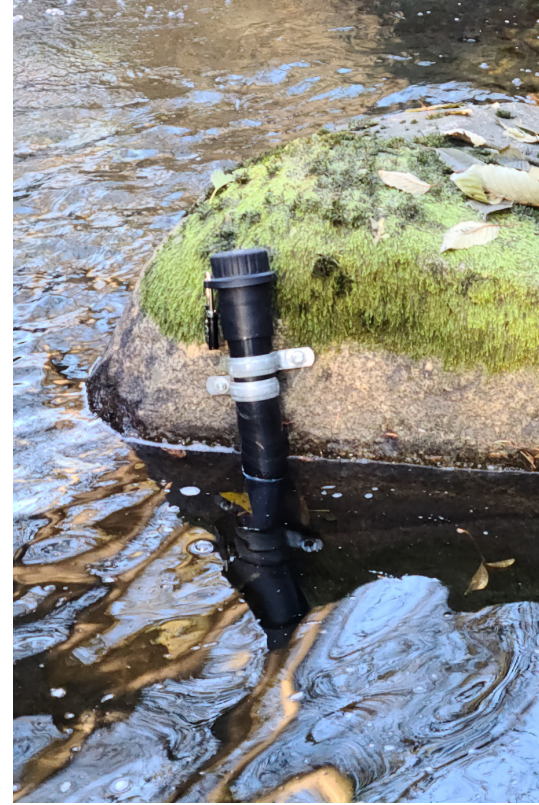
Photo: a conductivity logger installed in a North Vancouver creek
